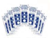
• WarmMark/ WarmMark Duo / WarmMark Long Run: besides indicating whether the temperature has exceeded the set limit, they also inform you of the exposure duration to excessive temperatures, so you can make a more precise assessment as to the possible damage caused to your products during such events. They can monitor temperature from -18°C to +37°C, with a sensitivity margin of +/- 1°C and 3 year shelf life from the production date.
