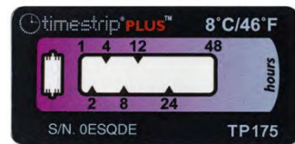
Timestrip Plus 175 8°C 19mm x 40mm 48 hour run-out window Activation blister on top For fridge, pharma shipments.
