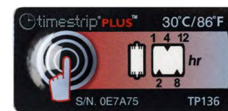
Timestrip Plus 136 30°C 19mm x 40mm 12 hour run-out window Activation blister on top For controlled room temperature.
