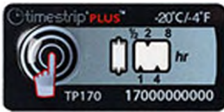
Timestrip Plus 170 -20°C 19mm x 40mm 8 hour run-out window Activation blister on top For dry ice shipments.
