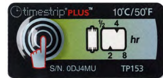
Timestrip Plus 153 10°C 19mm x 40mm 8 hour run-out window Activation blister on top For fridge, pharma ward use.
