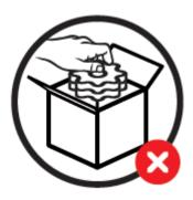
The parts must be handled with clean gloves since fingerprints could cause corrosion on the metal surface.
