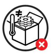
The parts must be packed at room temperature (neither too hot nor too cold) to avoid condensation. It is recommended the use of desiccant bags inside packaging to prevent any problem of condensation.
