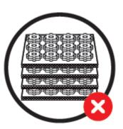
Avoid direct contact of the parts with organic materials (untreated VCI paper, wood, cardboard) that may contain humidity and/or acids.
